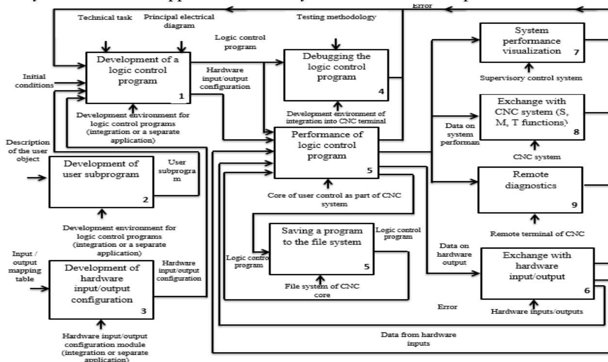
Figure 1. Functional model of logic control systems in IDEF o notation
