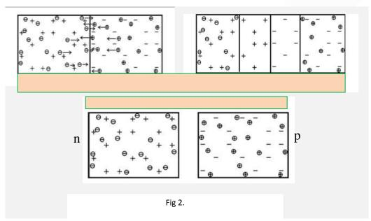
Photovoltaic effect in the p-n junction. The solar cell makes it possible to convert the energy of optical radiation directly into electricity, bypassing the stages of thermal and mechanical forms of energy. His work is based on the internal photoelectric effect in a semiconductor structure with a p-n-junction (heterojunction, Schottky barrier). The SC of the simplest design consists of two layers of different types of conductivity (electronic - n and hole - p) (Fig. 2).
