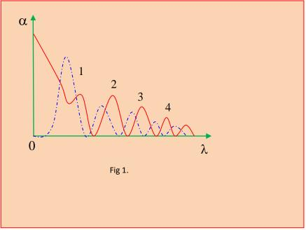
The dependence of the absorption coefficient Q(x) on the wavelength of the incident radiation  $\alpha(\lambda)$  is called the absorption spectrum (Fig. 1) [2]. Section 1 corresponds to its own absorption. The energy absorbed in section 1 is spent on breaking the valence bond and the transition of an electron from the valence band to the conduction band. To transfer an electron to the conduction band, it is necessary that the energy of the absorbed photon exceeds the band gap:
